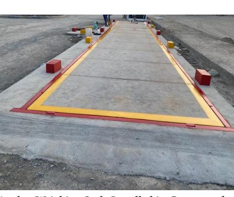
Analog Weighing Scale Installed in Customs of Spin Boldak
