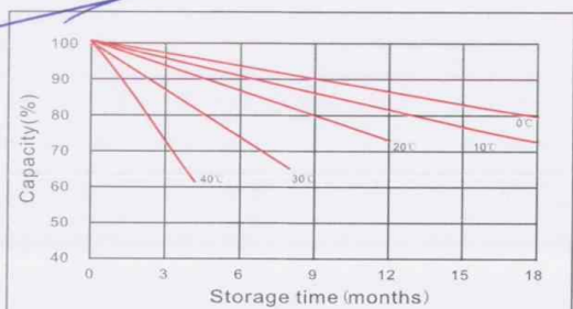
Curves of self discharge
